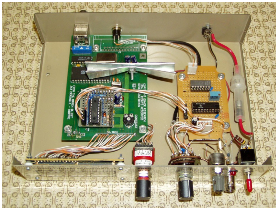
Figure 3: Internal View 1 Upgraded DigiVFO/DigiBrain
