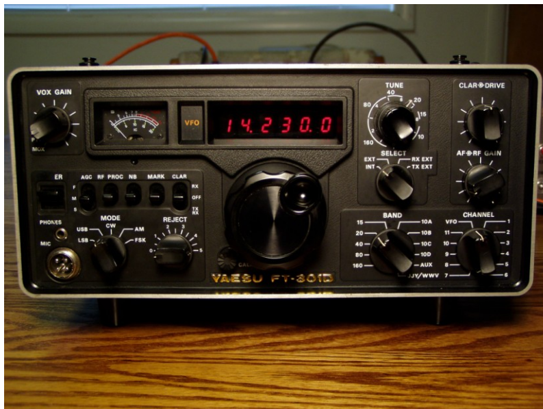
Figure 6: FT-301D with the new PB-1542B-R display installed
